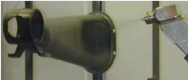
Figure 12: The robot painting the steering column with the automatically generated program. The black paint can be seen on the part.
