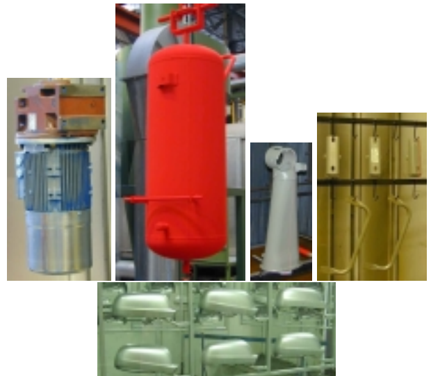
Figure 1: Examples of parts to be painted automatically: gearbox with motor, compressor tank, steering column of a truck, small parts on a frame, and rear view mirrors. The pictures show the parts in correct relative size.
