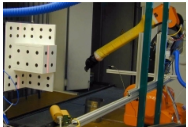
Figure 11: Painting cell with the calibration tool (left) and the camera (bottom front).
