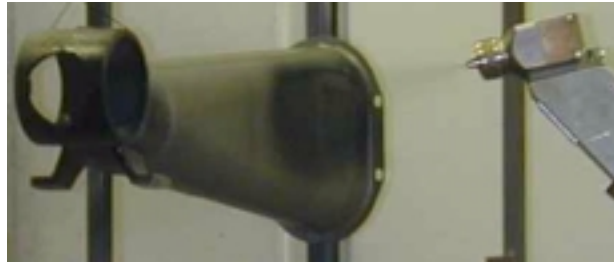
Figure 4: The robot painting the steering column with the automatically generated program. The black paint can be seen on the part.
