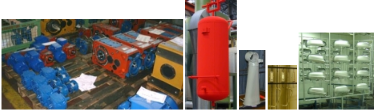
Figure 1: Examples of parts to be painted automatically: various gear boxes with motor, compressor tank, steering column of a truck, small parts on a frame, and rear view mirrors on a frame. The pictures show the parts in correct relative size.
